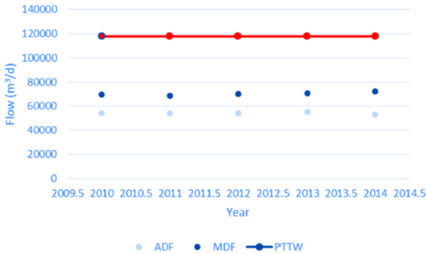
Figure 7-5 Kingston Central Water Treatment Plant- Water Taking
