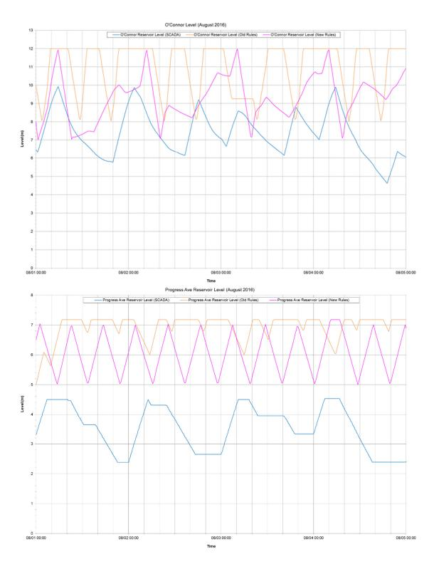
Figure 1-7a SCADA and Model Results on Tank Cycling Profile
