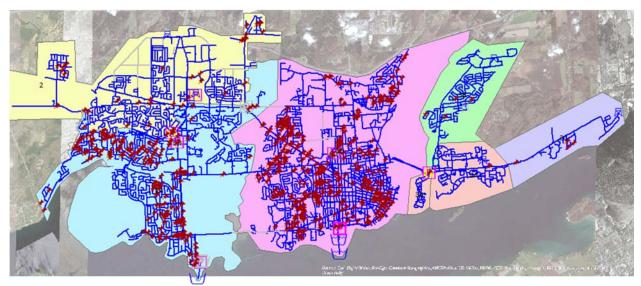
Figure 1-1 GIS Water beak layer within the Pressure Zones in the model (1998-2014)
