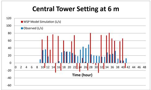
Figure E-6 Comparison of field observed flow and model simulation at Central Tower setting at 6 meters
