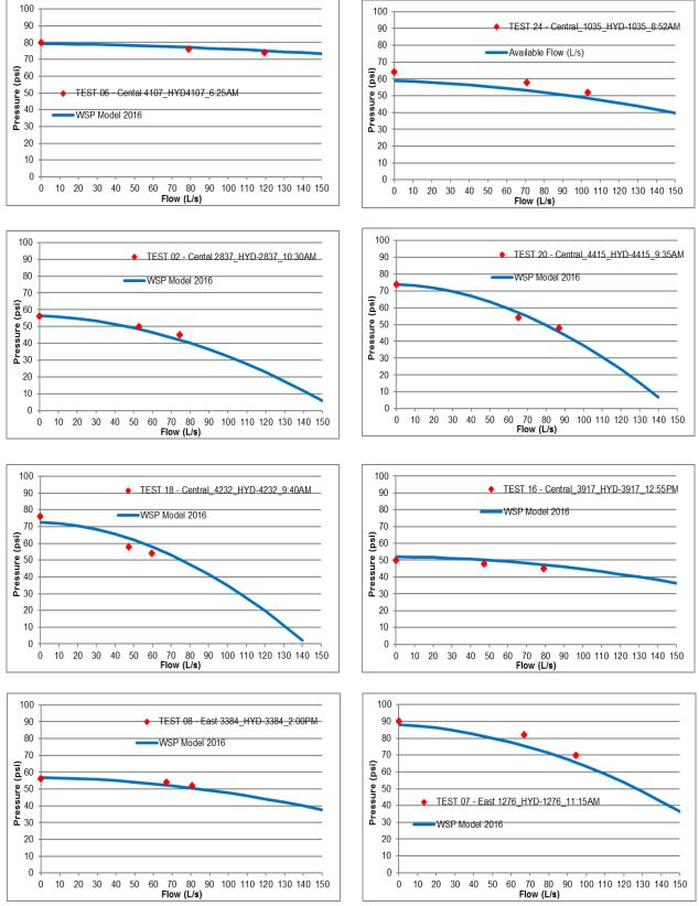
Figure E-3 WSP Model calibration – Hydrant Curves (1)
