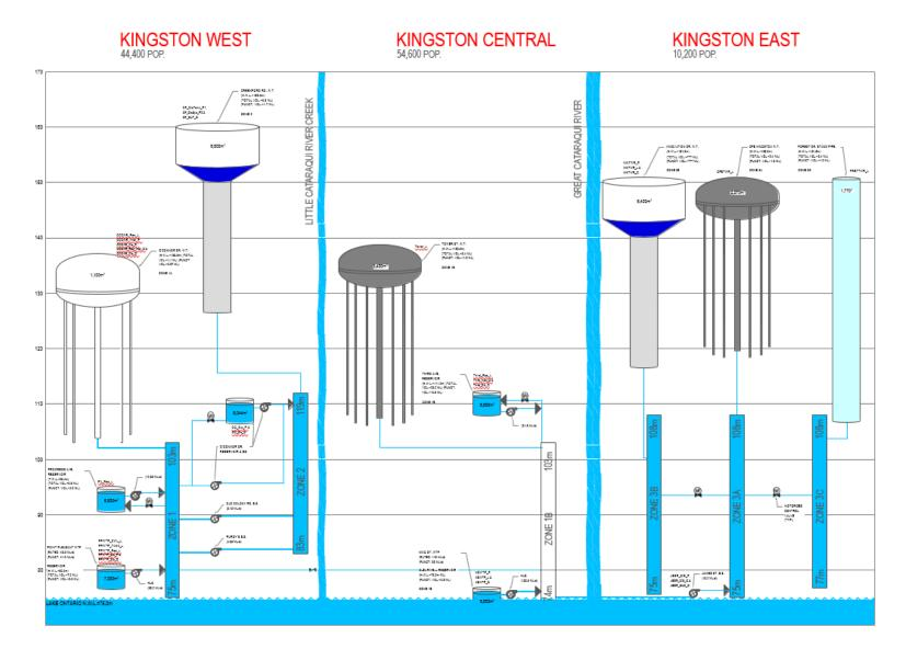
Figure E- 2 Kingston Water Distribution System Schematic
