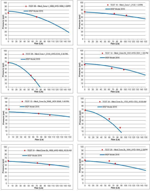
Figure E-3 WSP Model calibration – Hydrant Curves (2)
