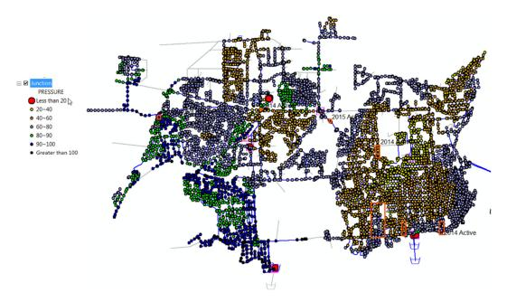
Figure 1-5 2015 interconnection\_ALT1 scenario PHD pressure without PRV/PSV control
