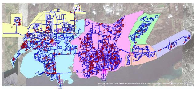
Figure 1-2 Leak repair/report tracking data within the Pressure Zones in the model (2011-2014)
