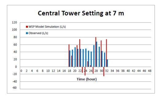
Figure E-7 Comparison of field observed flow and model simulation at Central Tower setting at 7 meters
