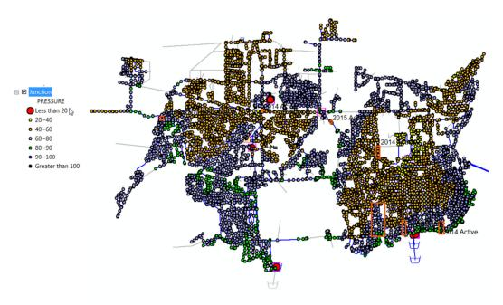
Figure 1-6 2015 interconnection\_ALT1 scenario PHD pressure with PRV/PSV control
