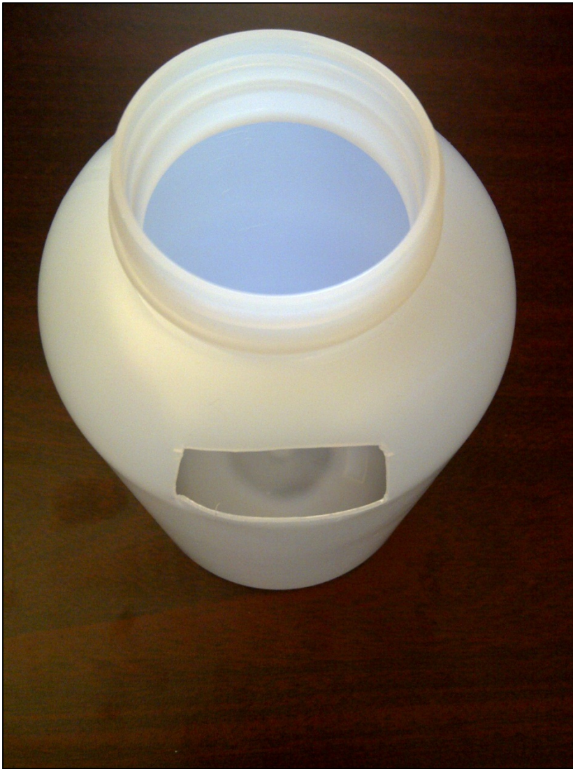
Figure 13: Transfer Bottle Modification for Low Flow Conditions
